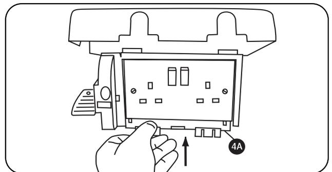
Once socketsafe is positioned in correct alignment with the wall socket, gently tighten the faceplate screws to fix socketsafe and the wall socket to the wall. Ensure there is a strong fix, allowing no movement of the unit when applying moderate force. Take care not to over tighten screws.
