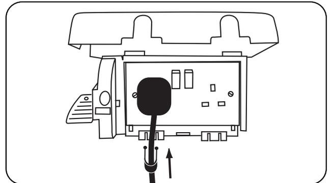
**Sometimes, without the cable ties in place, or when plugs with thicker than standard cables are in use, the socketsafe may not freely disengage of its own accord. In most cases, a gentle helping hand is all that is needed to guide the cover over the offending cable as the key is being turned.**
