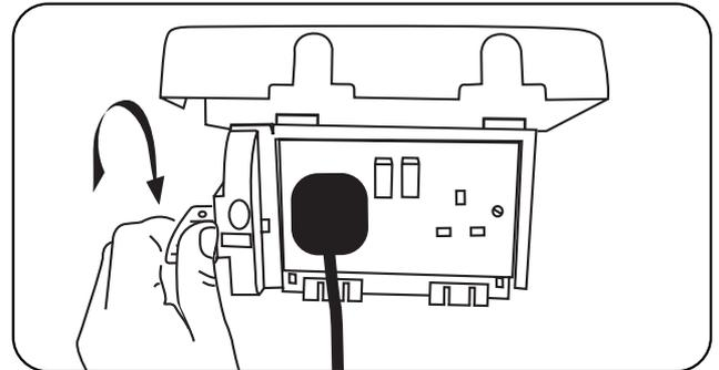
You can choose to fit the optional cable restraining ties. The cable ties keep the plug leads secure and prevent interference with the socketsafe cover when opening. Pinch the cable tie inwards and slide upwards into the slots as shown. Power the switch on and then gently close the cover.
